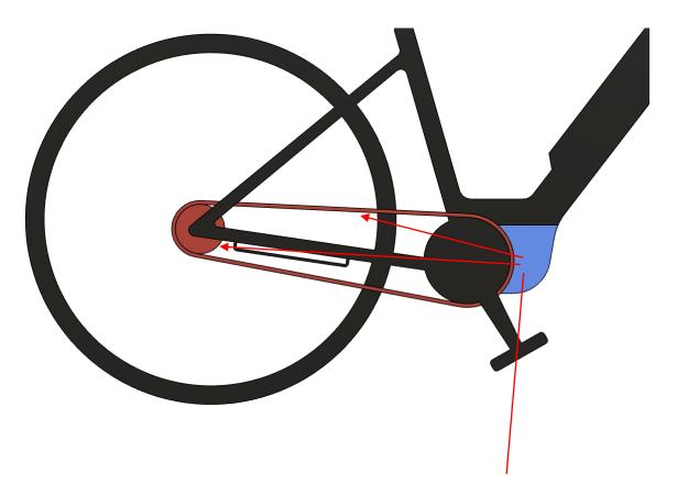
The standard torque power of a mid drive unit is between 80 - 110Nm, the same values are transmitted to the chain/belt and a shifting system.
