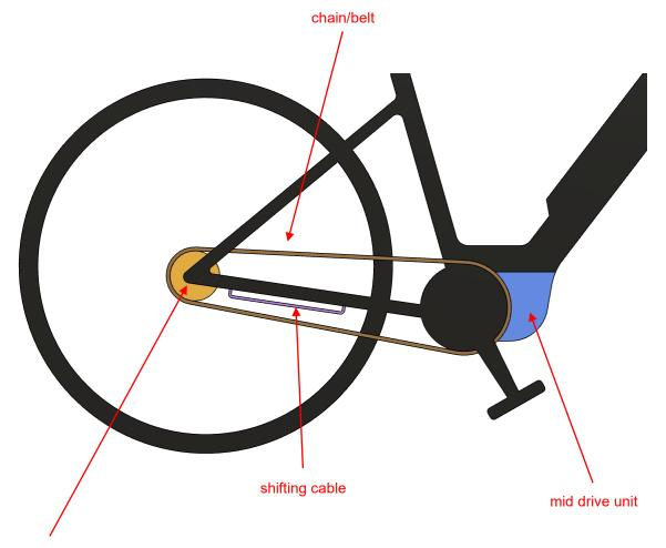
shifting system (rear derailleur or internal gear hub)
