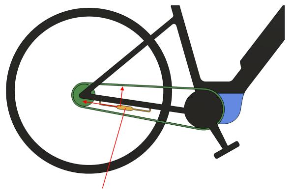
The gearsensor.com reduces torque power of the motor when the rider needs to shift up or down. As a result, there is no longer any pressure on the chain/belt and shifting mechanism. The rider can shift without any complications, in any situation.
