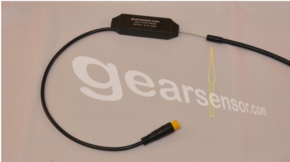
In below picture the inner cable is correctly fixed into the housing. Then adjust shifting system properly, and connect gearsensor.com to drive unit input.
