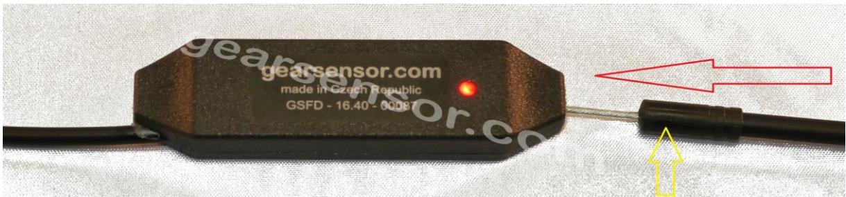
In below picture the inner cable is correctly fixed into the housing. Then adjust shifting system properly, and connect gearsensor.com to drive unit input.
